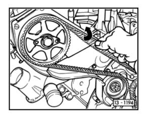
Check beltension by gripping belthalf-way between cam shaftsprocket and coolant pump.
