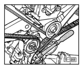
The toothed belttension adjustment is done by turning the tensioning rollerwith 8 mm hex-key wrench.
